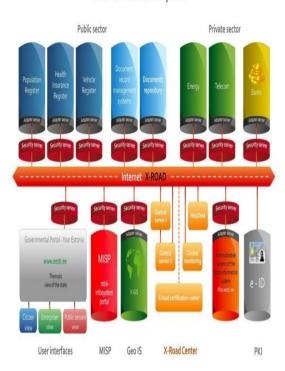
**Fig. 6.** Estonian Information System based on X-Road, adapted from the State Information Agency [16].
